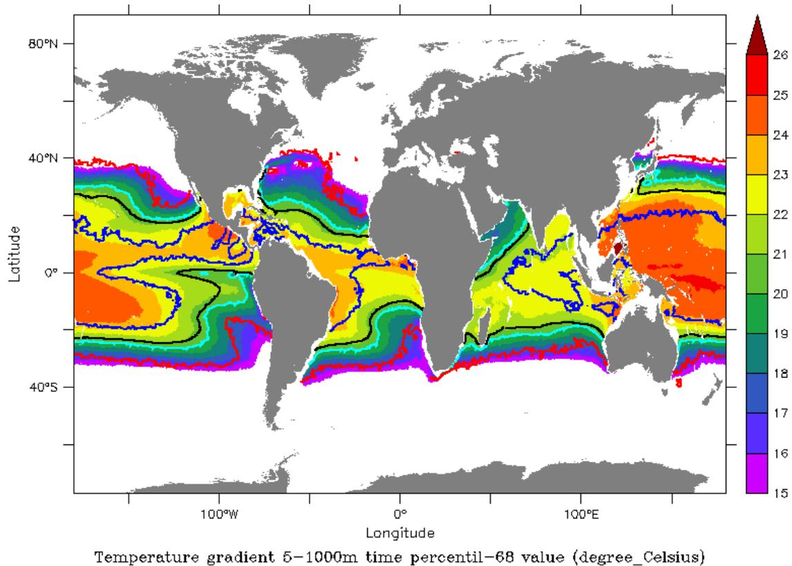
**Figure 3-15:** From G2V1 temperature monthly averages, computation of the 5-m to 1000-m differences. From time series of differences, plot of the percentile 68value for each grid point (in °C). The cyan isoline corresponds to the 20°C difference for this percentile. 20°C contour for the maximum (red), minimum (blue) and mean (black) fields are also plotted (see Figure 3-12 and Figure 3-13 for explanations).
