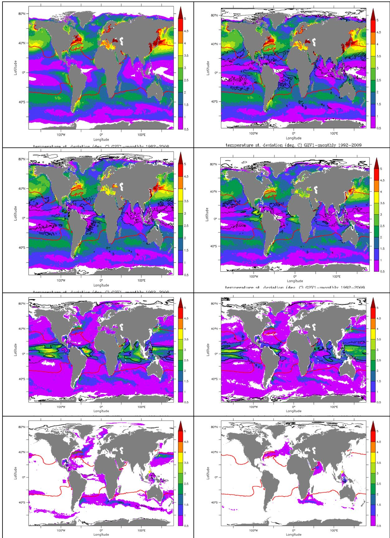
**Figure 3-9: G2V1 monthly temperature fields time varying statistics at level 1 (0.5-m, top left), level 5 (5.1-m, top right), level 12 (19.4-m, medium left), level 15 (30.9-m, medium right), level 24 (97-m, medium low, left), level 28 (147.4-m, medium low, right), level 40 (508-m, bottom left), and level 47 (1046-m, bottom right). The time standard deviation (in deg. C rms) is shaded. The Red isoline corresponds to the area where at least one**
